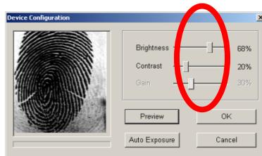
4. To let the system automatically determine optimal settings, place your finger on the reader and then click **Auto Exposure**. Hold your finger still while the settings automatically change incrementally. This may take several seconds. Once completed, place your finger on the reader again, and then click **Preview** to view the improvement of your fingerprint.
