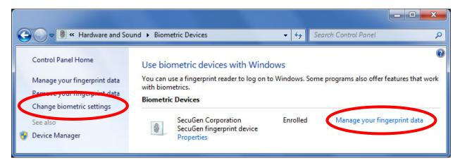
6. To use your fingerprint to logon to Windows, Biometrics should be turned on. If the SecuGen WBF device driver is properly installed, it will be turned on by default. To change the biometric settings, click on *Change biometric settings* from the Biometric Devices Control Panel (above).
