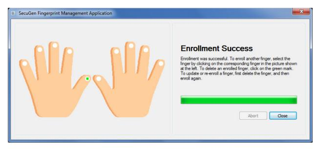
**Note**: If the tip of the finger is colored green, that finger has been successfully enrolled. To delete an already-enrolled finger, click on the green tip. After deleting, you can re-enroll that finger.
